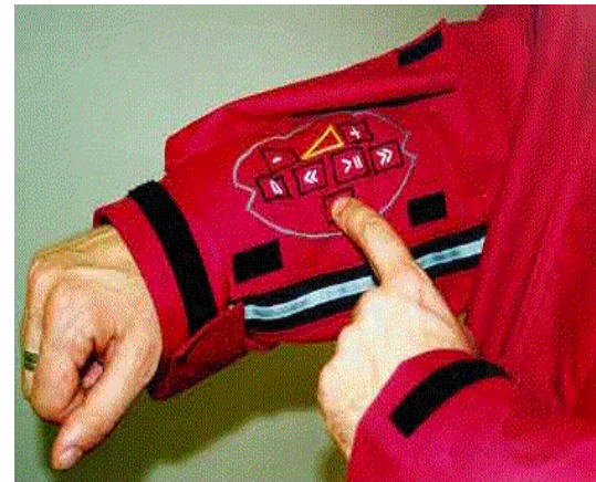
Wearable audio keypad incorporating Softswitch technology from WRONZ/Peratech.
